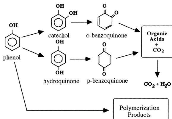
Fig. 5. Simplified reaction pathway of the phenol oxidation reaction.
