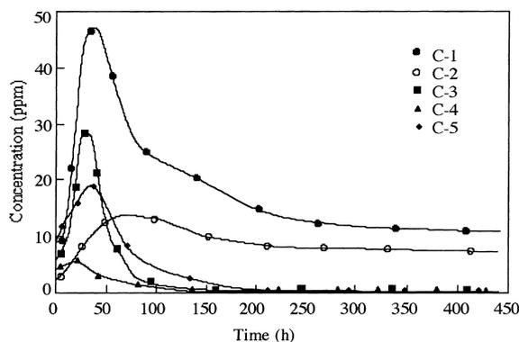
Fig. 6. Cu and Ni concentration profiles during the reaction process for the catalysts C-1 to C-5.
