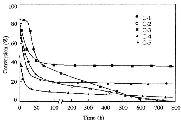
Fig. 3. Evolution of the phenol conversion for the catalysts C-1 to C-5.
