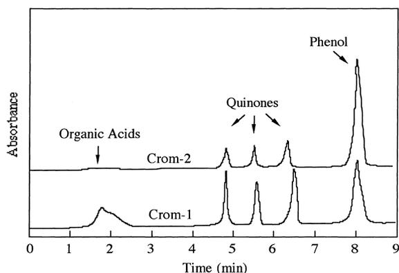
Fig. 4. Typical products detected by HPLC from copper C-1, C-3 and C-5 (Crom-1) and nickel C-2 and C-4 (Crom-2) catalysts.
