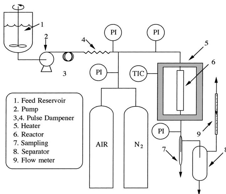
Fig. 1. Experimental setup for catalytic oxidation studies.
